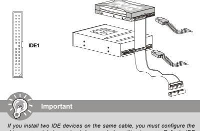
If you install two IDE devices on the same cable, you must configure the drives separately to master / slave mode by setting jumpers. Refer to IDE device's documentation supplied by the vendors for jumper setting instructions.
